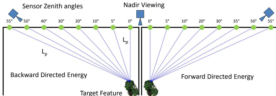
Figure 9. The translation based hyperspectral imaging goniometer (figure 4,5) data collection scheme used to collect SE590 and HSI system [11,12] images at each angle shown above in the backward and forward directions with reference to the target or feature. BRF and ANIF multi-angle signatures shown above were calculated at the shown sensor zenith angles at a sensor azimuth of  $352^0$  degrees.
