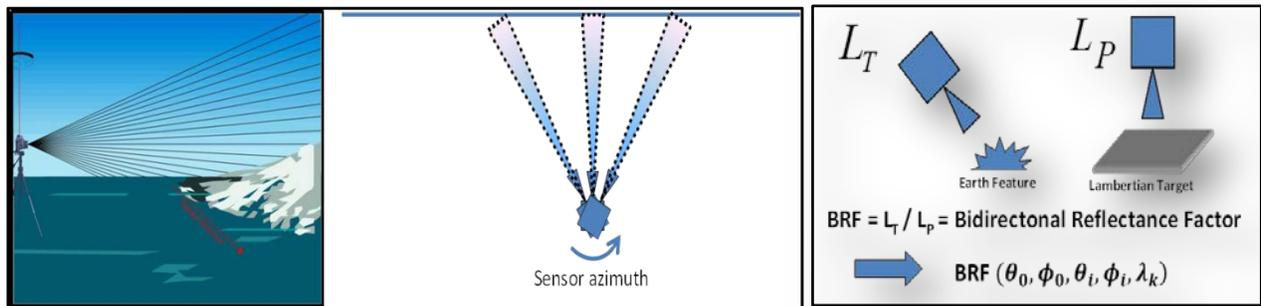
Figure 3. Operational multi-angle hyperspectral signature acquisition methodology used aboard a vessel as depicted above. The methodology allows for creation of signature libraries for use in developing BRF algorithms [8,9] used in airborne multi-angle flight missions in littoral zones. The approach uses sensor azimuth, sensor and solar zenith angles.
