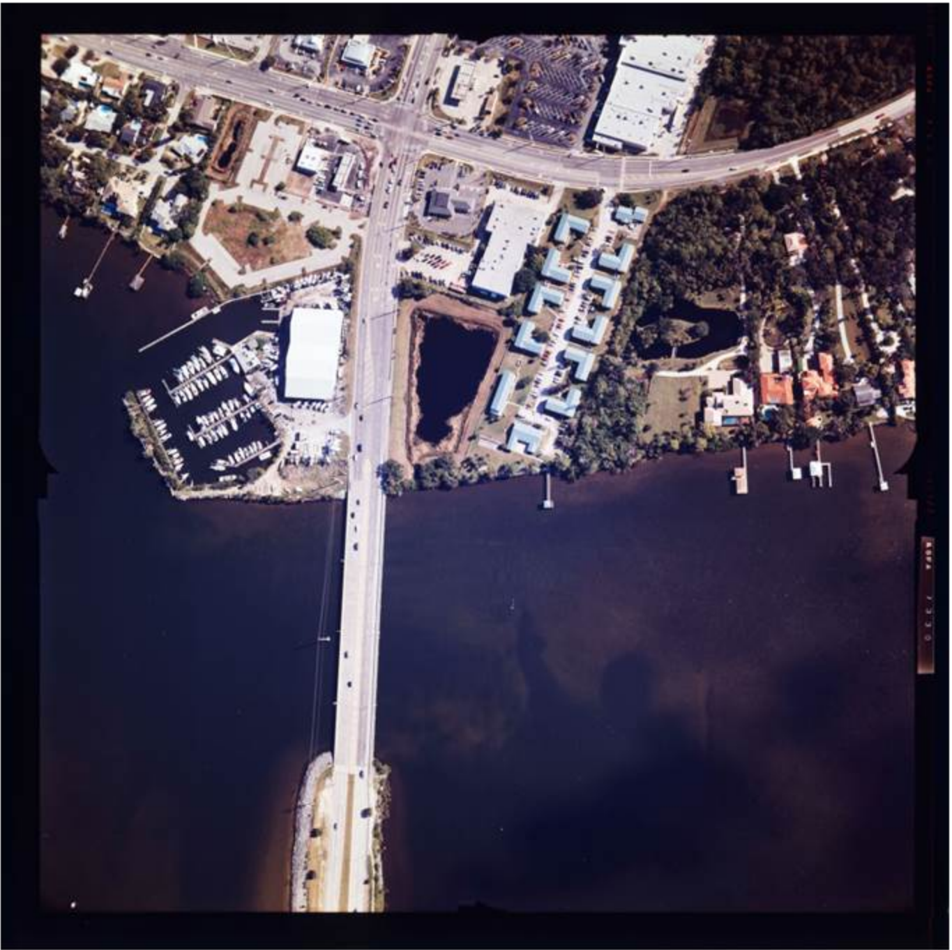
Airborne 255 megapixel 3 channel digital multispectral image along the Eau Gallie Causeway. Mapping camera flown at low Altitude using AGFA color negative film and Scanned using a Scanatronics optical glass plate for elimination of newton rings. Image Collected By Dr. Bostater.
