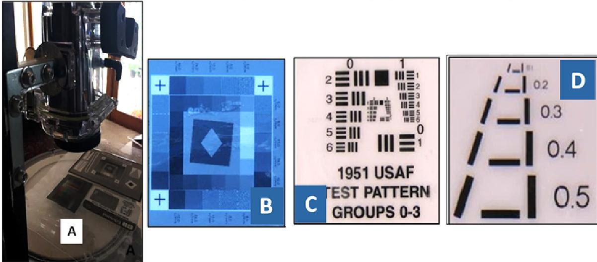
Figure 5. Image showing the floc multispectral camera system (A) and camera calibration targets used for focusing the camera before deployment from a vessel (images B, C, D) and for determination of effective pixel size resolution when viewing the illuminated circular LED light guide.
