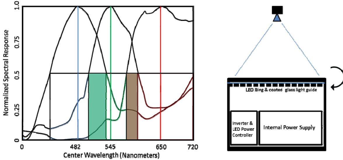
Figure 3. Normalized spectral response curves (left) of the multispectral camera used to test the *in-situ* subsurface spectral imaging of flocs. The submersible floc camera system is depicted (right) showing the components contained within a watertight submersible case for deployment up to 3.8 atmospheres (39 m). The system can image vertically or horizontally when deployed at the water bottom.
