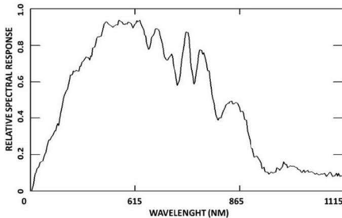
Figure 4. The spectral response curve of the LED light guide after the active light passes through the anti-reflective coated wave guide within the underwater housing. The measured signature was obtained with a SE590 high radiometric sensitivity and narrow band solid state spectrograph at the height above the light guide where the spectral camera collects imagery of the colloidal particulates.
