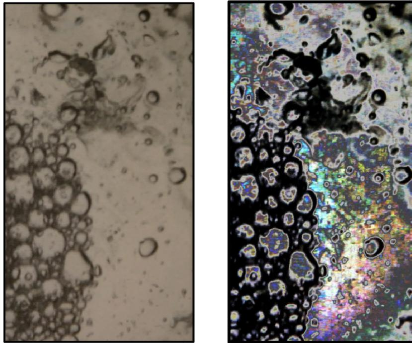
Figure 7. Multispectral mage acquired during deployment of the floc camera system. Small bubbles are observed as the system enters the water. The same image (right) is a contrast stretched image of bubbles at the surface of the circular LED light guide. The ability to discriminate small particles such as bubbles allows for independent particle size calibrations
