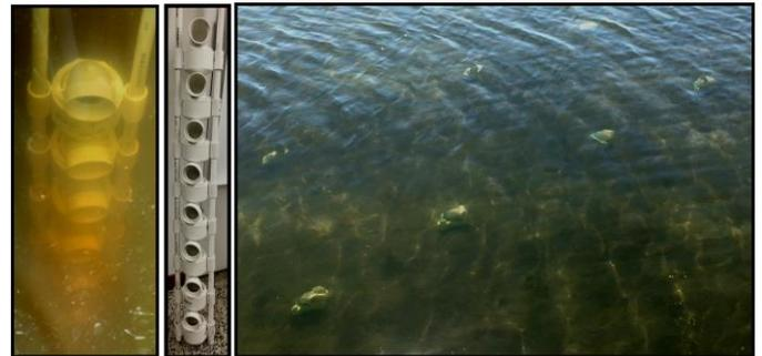
Fig. 3. Vertical array of eight horizontal flux sondes in the field (left), the center image shows the array of sondes in the lab before field deployment. The right image shows the horizontal flux sondes located in a two dimensional array (4.5 x 2 m).
