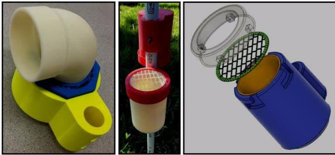
Fig. 1. Fluid mud sondes created using 3-D printers based upon computer aided designs originally described in Bostater and Yang (2014) using off-the-shelf PVC components.
