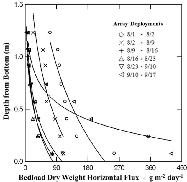
Fig. 4. Fluid mud vertical array profiles results from sonde deployments from August through September 17, 2017.
