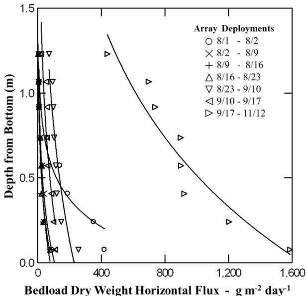
Fig. 5. Fluid mud vertical array profiles results from sonde deployments from August through November 12, 2017. The influence of hurricane Matthew caused a 4 fold increase in the movement of particulates within the lutocline at the water bottom at  $z=0$ .
