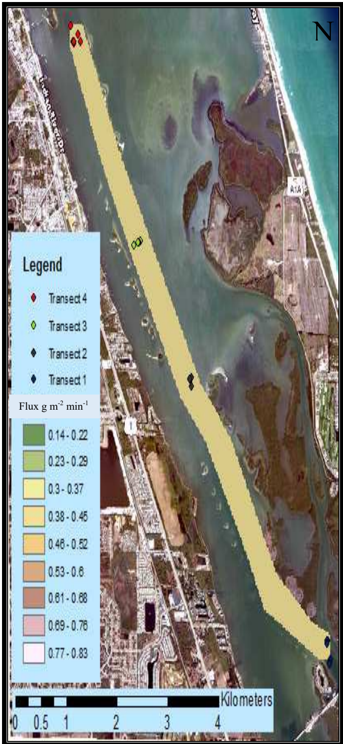
Figure 4: During-dredging dry weight fluxes ( \text{g m}^{-2} \text{min}^{-1} ) in-between the Wabasso Bridge and South side of the Sebastian Inlet. Channel cross sections are labeled from South(1) to North(2). (Multispectral image: Courtesy of Digital Globe)
