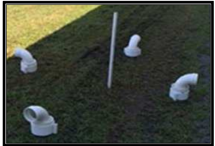
Figure 2: Mock directional orientation of the horizontal and vertical sonde set up at each location.
