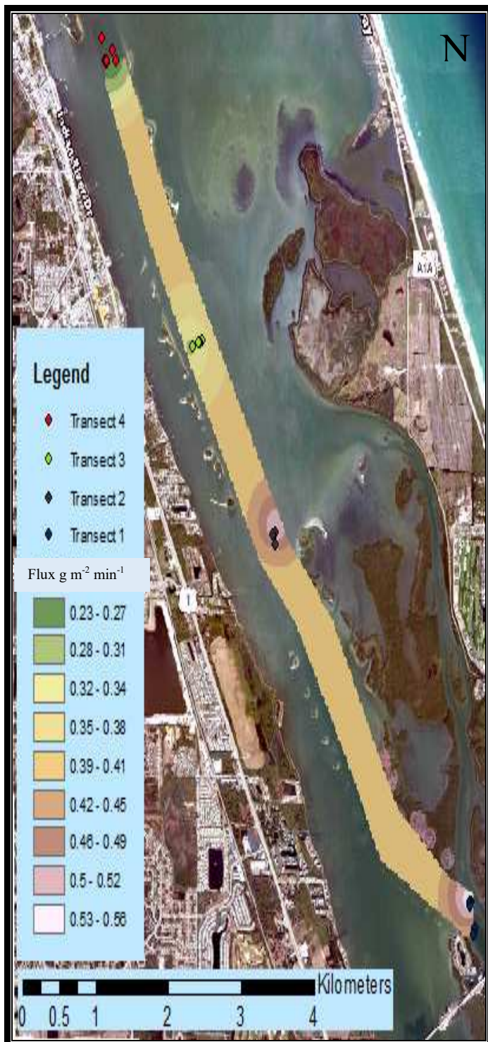
Figure 5: After-dredging dry weight fluxes ( \text{g m}^{-2} \text{min}^{-1} ) in-between the Wabasso Bridge and South side of the Sebastian Inlet. Channel cross sections are labeled from South(1) to North(2).
