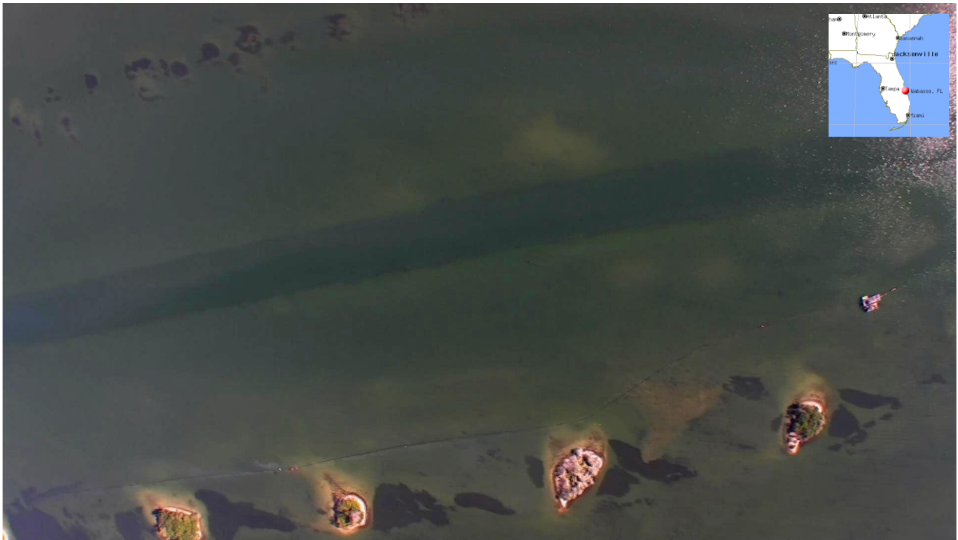
Airborne 3 Channel Multispectral (RGB) Image Display. Collected Friday Jan. 30, 2015 by C. Bostater. Snapshot MS image acquired between 10-11:45 AM at 760 m altitude. FIND Dredge Area, Intracoastal Waterway near Duck Point opposite North Oyster Island, Florida, Indian River Lagoon (~N 27.775094, W, -80.4436386).
